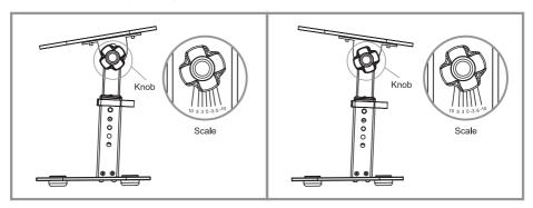
Loosen the knob you can adjust the angle (adjustable angle -10°,-5°,-3°,0°,3°,5°,10°). A 10°forward through to 10°backward tilt range allows you to set the optimum speaker face angle for each speaker set-up.
