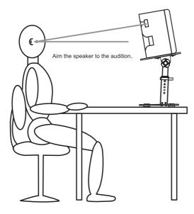
The tilt range is from -10°to 10°(adjustable angle -10°,-5°,-3°,0°,3°,5°,10°). According to your own height and speaker stand height, you can adjust the angle and height as above rules.
