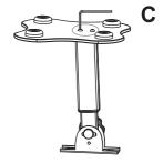
Secondly, use the hexagon wrench (6) to fasten two hexagon thumbscrews (5) on the base plate (4).
