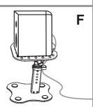
Finally, put the speaker cable along with cable casing and then through the cable clip(7).
