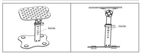
Press the marble you can adjust the height. Height adjustable allow you set-up in four-level which can suitable for most consumer.
