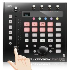
1. Plug in the wireless USB dongle into your PC/Mac USB port and then switch on the power of your PlatformNanoAir device.
