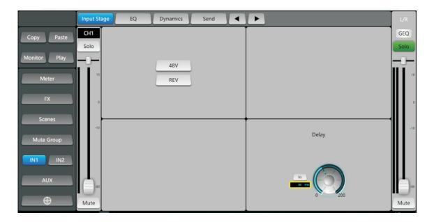
5. Select Input Stage tab, go to input channel settings page, current channel 48V, REV (phase) and Delay parameters can be controlled.
