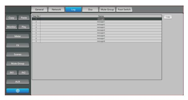
17. Select log option to enter system log page, which saves the last 10 boot records, use Copy button to copy the log information to an external USB flash disk (requires inserting a USB flash disk).
