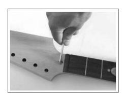
tightening the truss rod adjustment nut that protrudes from the base of the headstock just above the nut. A "back bow" or "hog-back" can be removed by loosening the nut. Great care should be taken with truss rod adjustments where as little as 1/4 of a turn can vastly alter the shape of a neck. A broken truss rod of course means a costly replacement.
