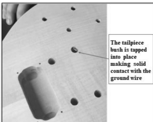
Installing the tailpiece bushing may be done with a plastic headed mallet or place a small piece of wood on top of the bushing to prevent damage and tap the bushing in place with an ordinary hammer. Now screw the tailpiece mounting screws back into
