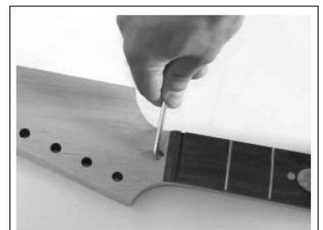
tightening the truss rod adjustment nut that protrudes from the base of the headstock just above the nut. A “back bow” or “hog-back” can be removed by loosening the nut. Great care should be taken with truss rod adjustments where as little as 1/4 of a turn can vastly alter the shape of a neck. A broken truss rod of course means a costly replacement.
