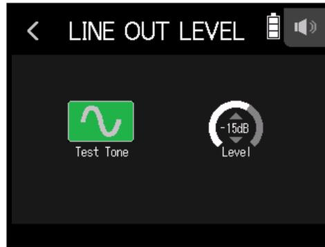
While checking the audio level meter of the other device, adjust the audio signal level so that it never exceeds -12 dB.
