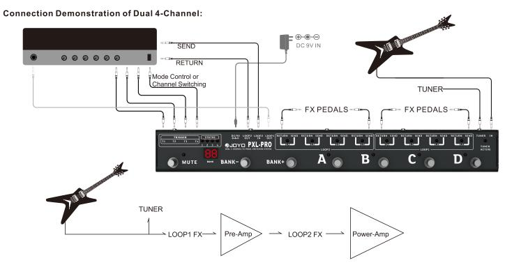
2, Under Bypass state, all channels of LOOP1/2 are directly connected without signals passing through effect pedals. While under Non-Bypass state, the signals flow through chosen channels of LOOP1/2.
