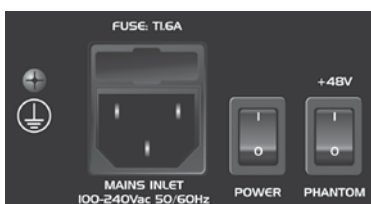
Fig. 2.16: Voltage supply and fuse
