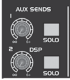
Fig. 2.6: AUX SEND controls of the main section
