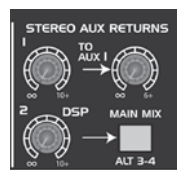
Fig. 2.9: Stereo aux return controls
