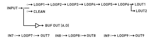
Guitar signal feeds into GEC9 input (NBUF IN or BUF IN), enters series LOOP1~LOOP6 when MUTE switch is off, then outputs from LOUT1 and LOUT2. If MUTE is on, the signal outputs directly to CLEAN jack. The BUF OUT jack always outputs buffered input signal.
